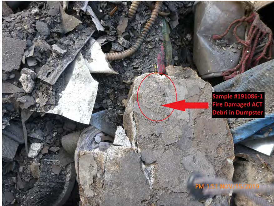
Photograph 3: November 15, 2019, at approximately 1:51 PM - View of fire damaged acoustic ceiling texture (ACT) debris in the 16 cubic yard dumpster. The ACT debris was sampled and later determined to contain 2% Chrysotile Asbestos. The ACT debris was in a dry condition.
