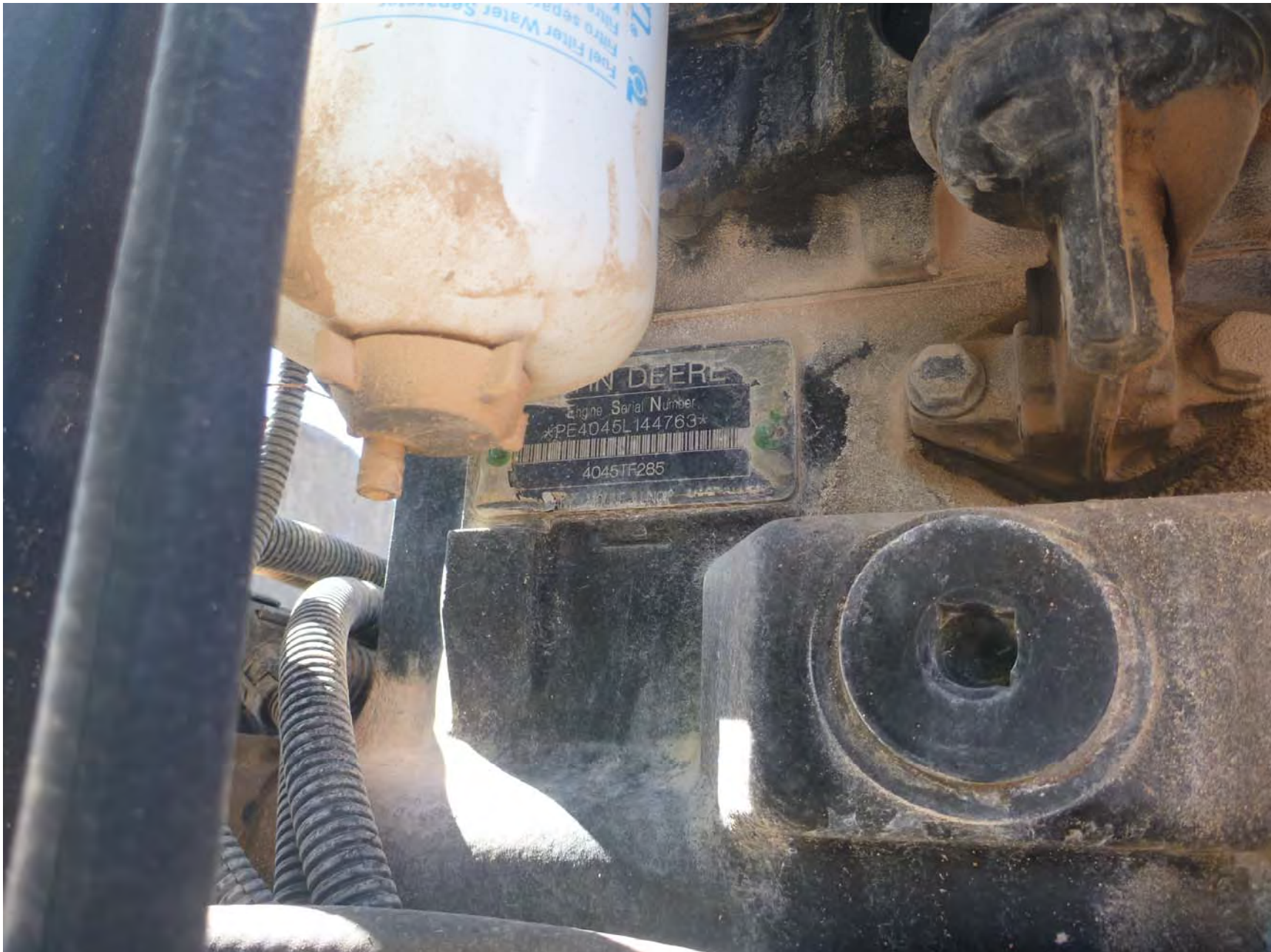
Photograph 15- Serial plate of Continuous Duty Diesel Engine (Water Pump) (EU: C07) depicting model number: 4045TF285 (See Attachment 19). Photograph by Canon Liddell.
