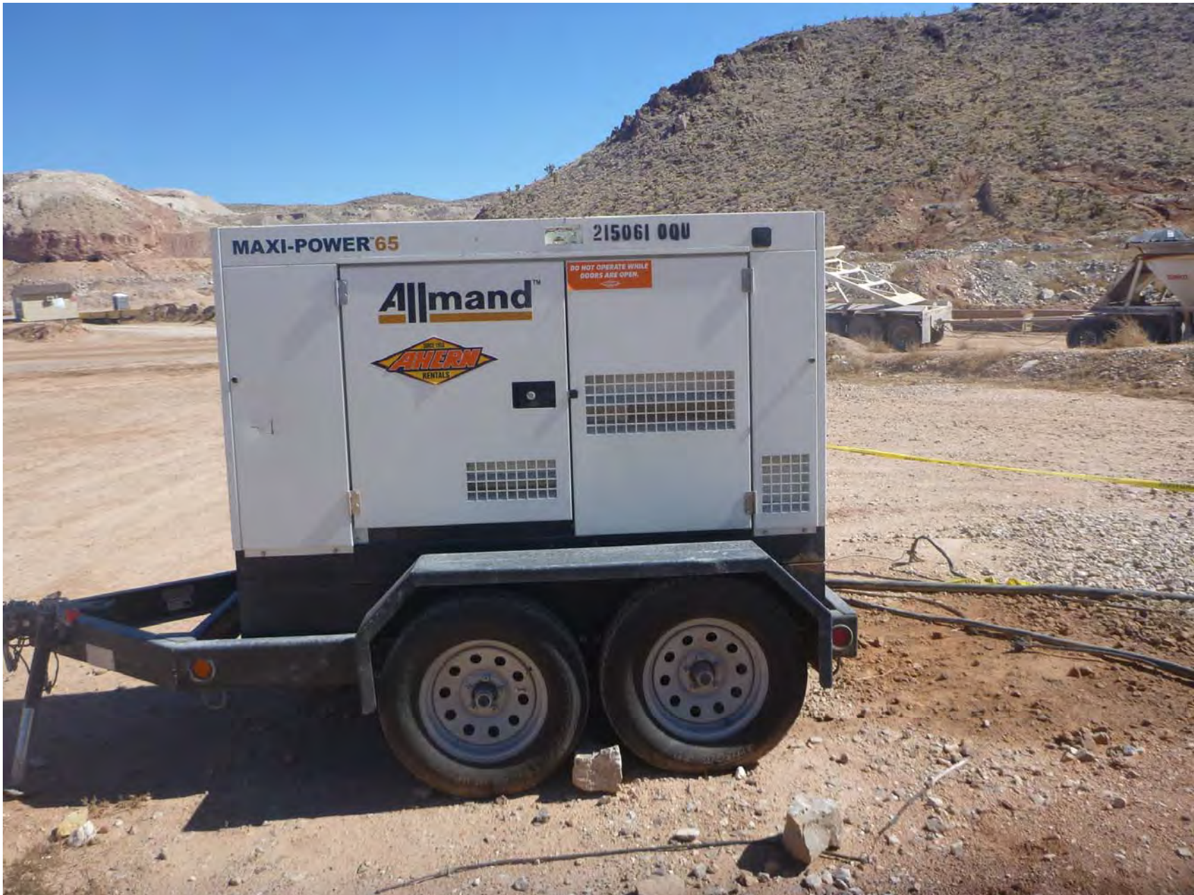
Photograph 11- Continuous Duty Diesel Engine (Generator) (EU: C08) [Office]. Photograph by Camon Liddell.
