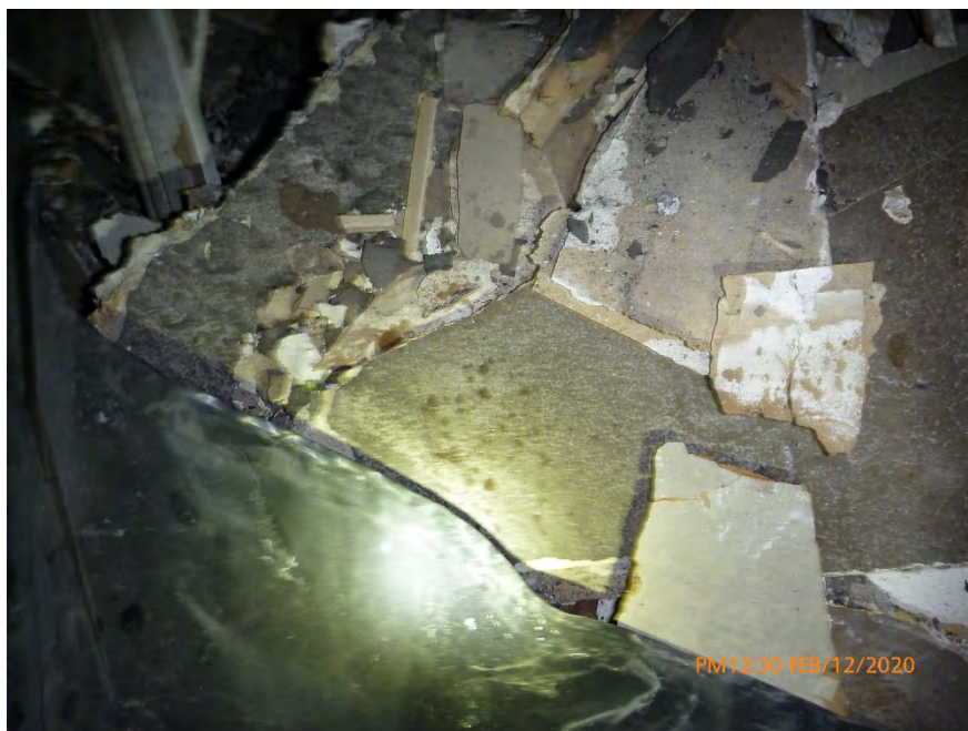
Photograph 31: February 12, 2020, at approximately 12:30 PM - View of textured drywall in a debris pile inside the north room of Unit 3. The material was sampled and later determined to contain 2% Chrysotile Asbestos by the point count method using polarized light microscopy. The material was in a dry condition with no evidence of moisture.
