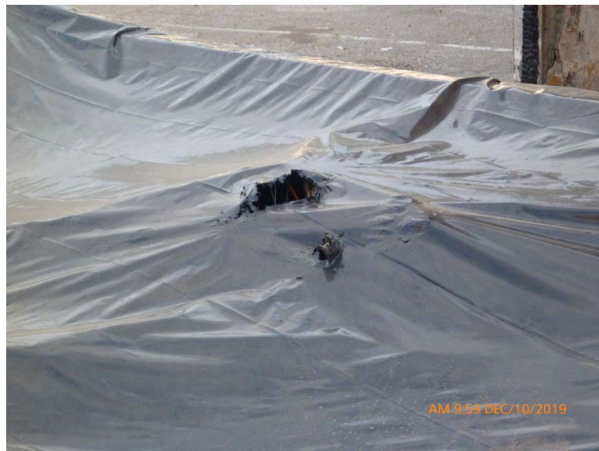
Photograph 29: December 10, 2019, at approximately 9:59 AM - View of the 16 cubic yard dumpster which contains ACWM. The dumpster is no longer sealed.
